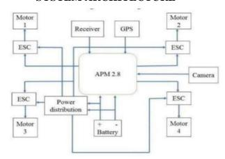
Fig -1: System Architecture Diagram
