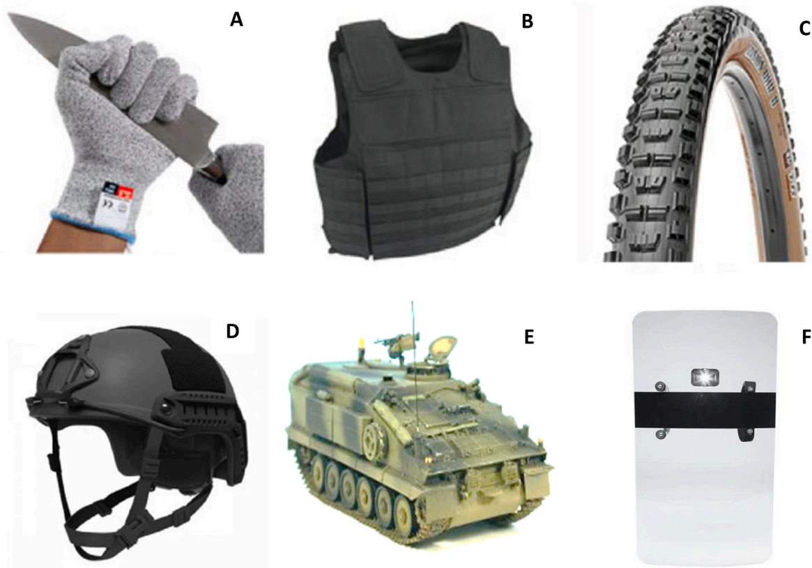
Fig. 3. Applications of Aramid and UHMWPE fibers in ballistic protection (Open source images) (A) Cut resistance Gloves, (B) Bullet Proof Vests, (C) Tyres, (D) Defence Helmets, (E) Vehicle Armor's, (F) Riot Shields.
