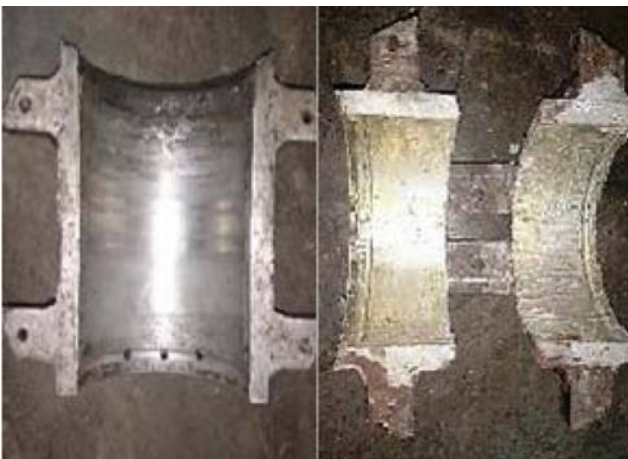
Figure 1 An effect of metal to metal contact
