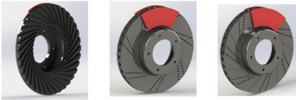
Figure 6 Discs with curved vanes, curved vanes with holes, and curved vanes with holes and slots (see online version for colours)
