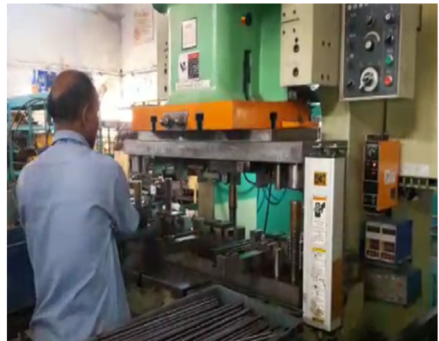
Fig. 19 Experimental setup of combination tool
