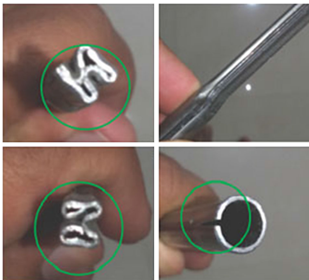
Fig. 5 Variety of defects observed
