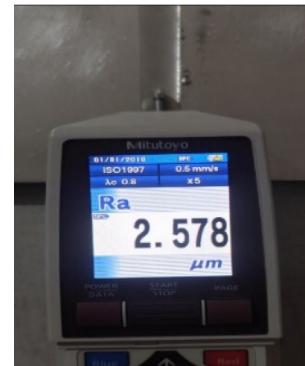
(b) Measurement of roughness of weld using roughness tester for experiment number 1
