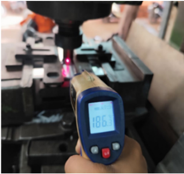
Fig. 4 Recording of Temperature using infrared thermometer during friction stir welding
