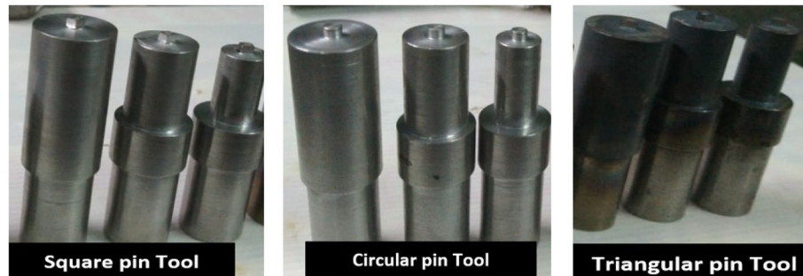
Fig. 1 Friction Stir Welding (FSW) tools with different pin profiles – square, circular, and triangular
