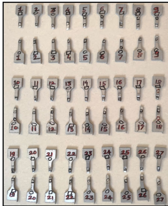
Fig. 4 Fractured tensile specimens of friction stir welded AA3103 joints after ASTM E8 testing
